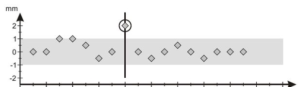
Figure 2b. Simulation field size: deviation between the set and measured positions for one of the wires delineating the simulation field set to 10 x 10 cm size (Oldelft).
