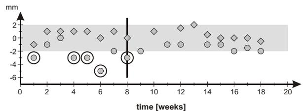
Figure 2c. SSD: deviation between source-to-skin distance indicated by the mechanical device (front pointer) and by the light scale (for 100 cm - circles, 80 cm - diamonds) (Ximatron).
