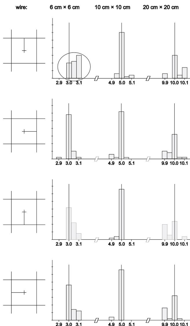
**Figure 3.** Simulation field size - histograms of measured values (set values indicated with vertical lines). The results are all within tolerance limits ( $\pm 1$  mm for each wire). However, some trends may be observed - for example for small field sizes (6 cm square field) one of the wires seems to be systematically misplaced (marked by an ellipse), which suggests the need or adjustment.
